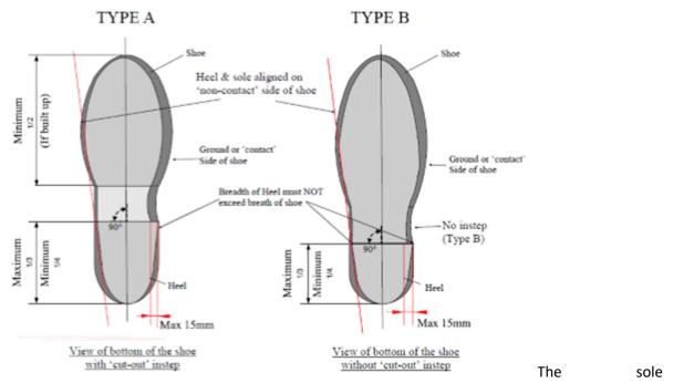
"structure" (which includes the structure of the heel) may be metal but the sole plate must not be metallic, the minimum thickness of the non-metallic plate is 6.5mm. See illustration below.
